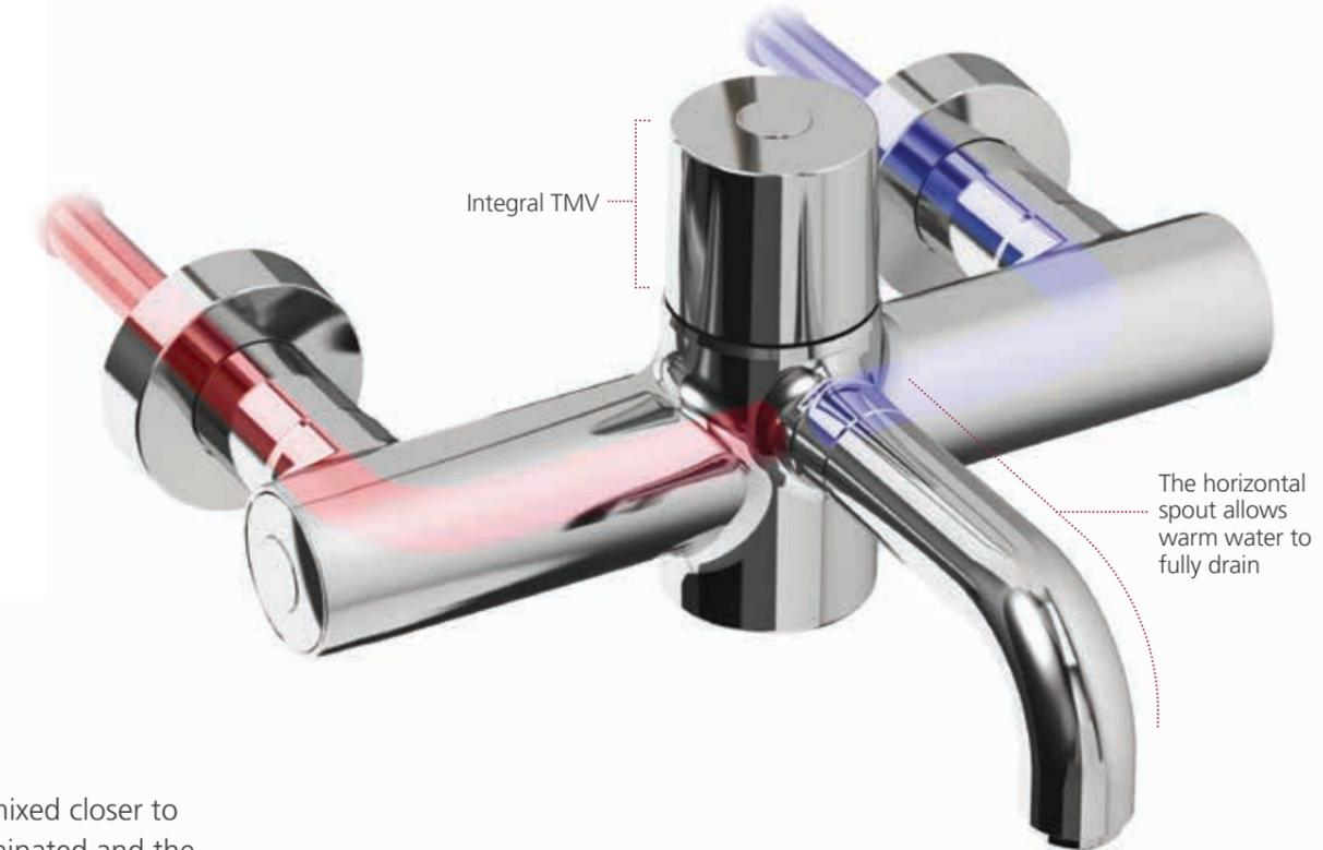
The Markwik21 integral thermostat enables water to be mixed closer to the point of discharge. The 'dead leg' of cold water is eliminated and the volume of mixed water is reduced, minimising areas of warm water which provides the ideal conditions for bacteria to grow
